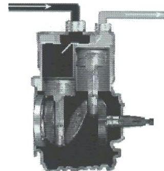
*Low pressure refrigerant gas leaves the evaporator and is drawn in by the compressor. Compressing the refrigerant raises its pressure and its temperature.*
