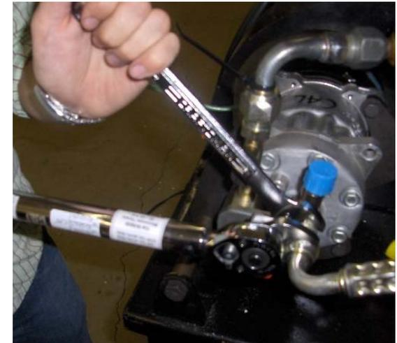
Tighten connection with proper torque.
