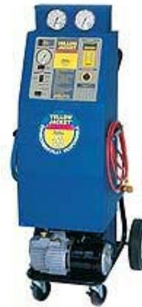
*To remove the refrigerant from the air conditioning system, you have to recover it, with a refrigerant recovery system. Never release the refrigerant to the atmosphere!*
