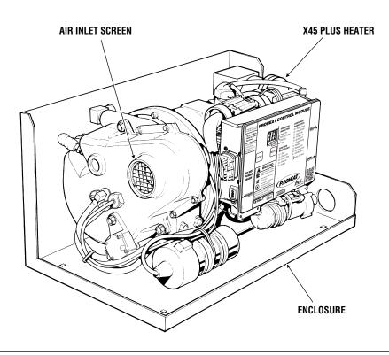
Figure 5-2. X45 Plus Heater and Enclosure
