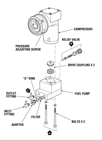
Figure 4-8. Compressor / Fuel Pump Assembly
