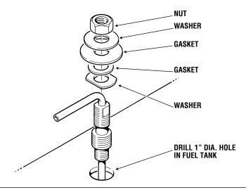
Figure 2-44. Drill Hole in Tank
