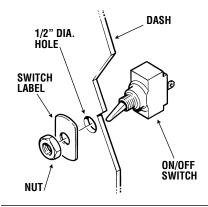
Figure 2-22. ON/OFF Switch Assembly
