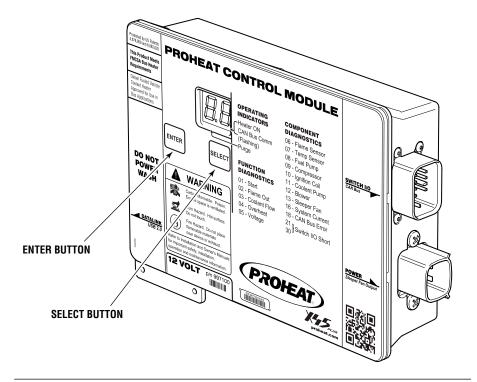
Figure 4-1. PCM – Mechanics Mode
