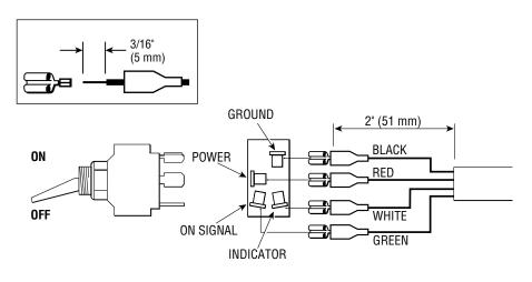
Figure 2-23. ON/OFF Switch Connections
