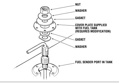
Figure 2-43. Blank Fuel Sender Port
