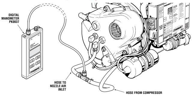
Figure 5-13. Air Compressor Pressure Test Procedure
