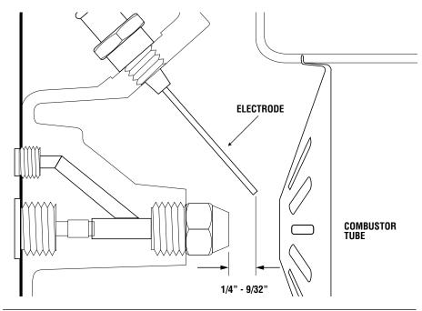
Figure 4-24. Electrode Gap Detail
