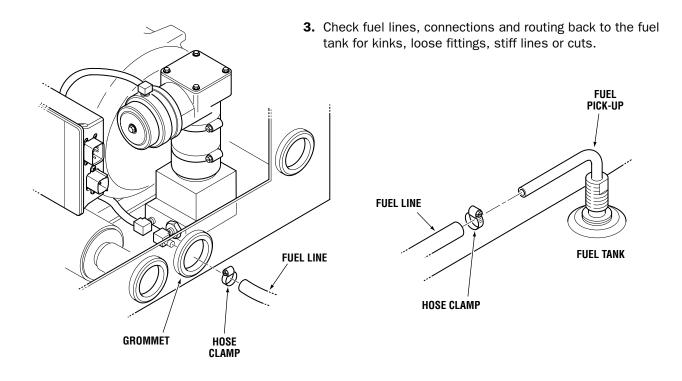
Figure 4-14. Check Fuel Lines, Connections and Routing
