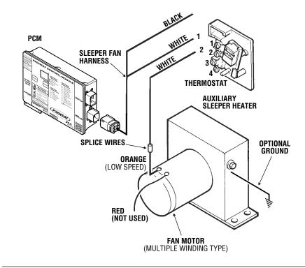
Figure 2-36. Auxiliary Sleeper Heater Installation
