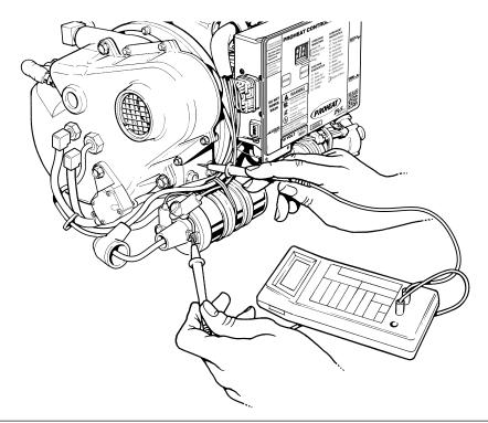
Figure 4-19. Check Coil Voltage
