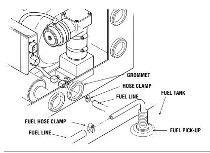
Figure 2-47. Fuel Line Connection Detail
