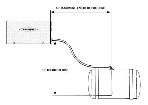
Figure 2-40. Fuel Supply Height Requirement
