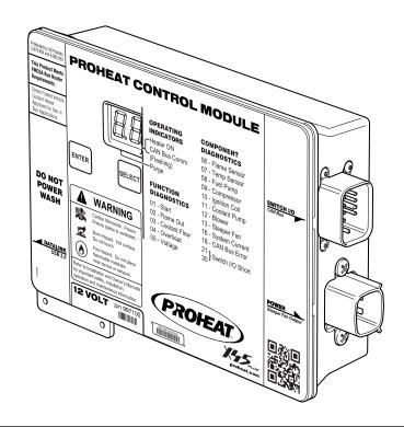
Figure 3-2. LED will light to indicate a problem. Switch or timer indicator light will flash to indicate the diagnostic code (page 4-3)
