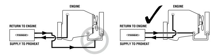
Figure 2-15. Correct Return Line Plumbing
