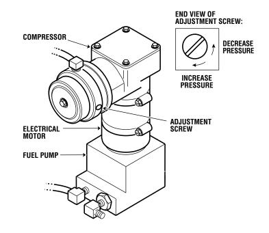
Figure 4-21. Compressor / Fuel Pump Assembly
