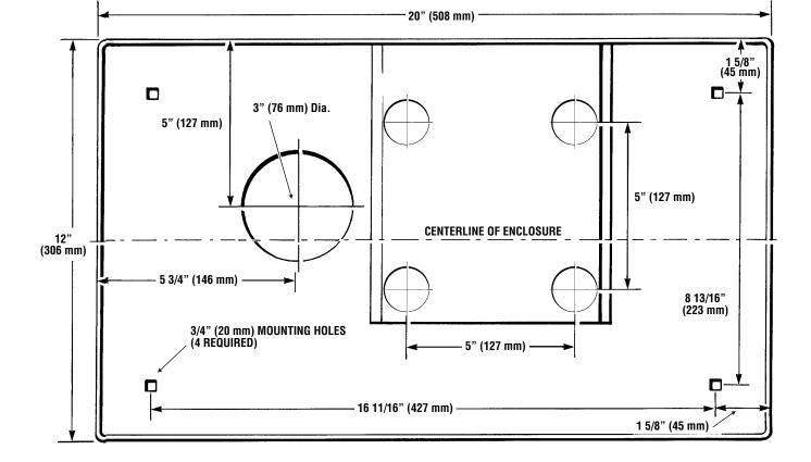
Figure 2-9. X45 Plus Enclosure Base Dimensions
