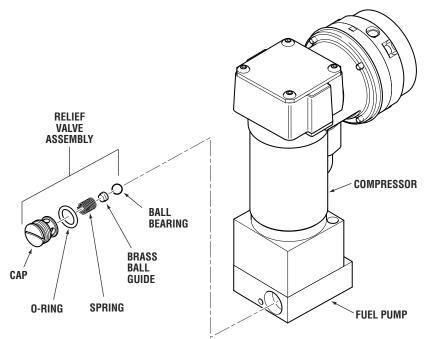
Figure 4-12. Pressure Relief Valve
