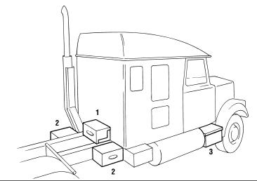
Figure 2-2. **Recommended Mounting Positions**
