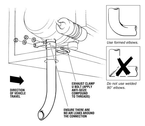
Figure 2-11. Exhaust Pipe
