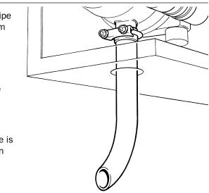
Figure 5-3. Exhaust Pipe
