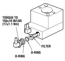
Figure 5-8. Fuel Filter Components
