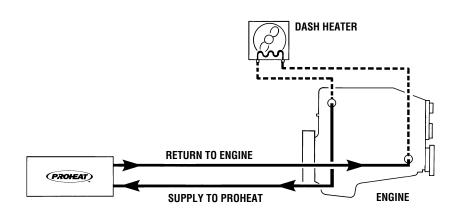
Figure 2-14. Engine Heat or Supplemental Heat
