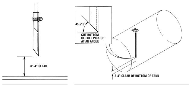
Figure 2-45. For some situations where the fuel pick-up is too far from the bottom of the tank, an extension from left over fuel line can be added.
