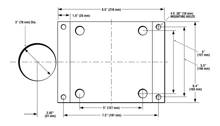
Figure 2-10. X45 Plus Mounting Plate Dimensions & Exhaust Hole
