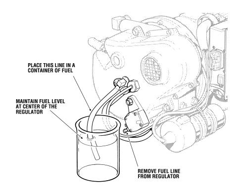
Figure 4-7. Eliminating Fuel Pump and Regulator from System
