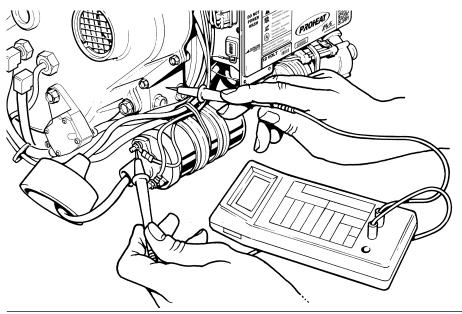
Figure 4-30. Heater Voltage Measurement
