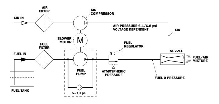
Figure 3-6. Fuel Delivery Theory of Operation
