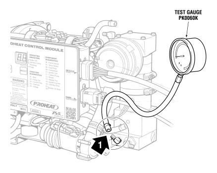
Figure 4-16. Remove Test Gauge
