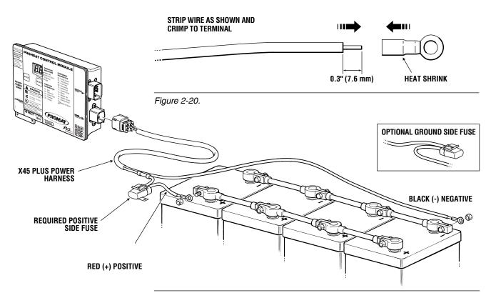
Figure 2-21. Power Connection to Battery.
