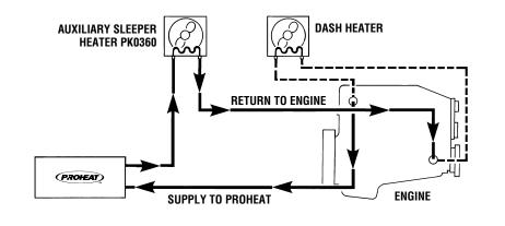
Figure 2-16. Engine and Sleeper Heat
