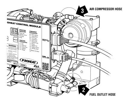
Figure 4-17. Reconnect Fuel Lines and Air Hose
