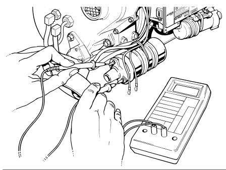
Figure 4-36. Ignition Coil Test
