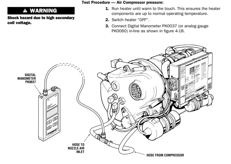
**Check Air Compressor Pressure and Operation**
