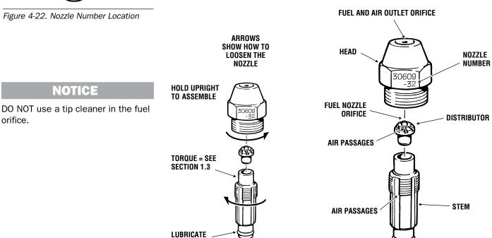
Figure 4-23. Fuel Nozzle Assembly
