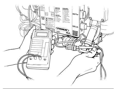
Figure 4-37. Coolant Pump Test
