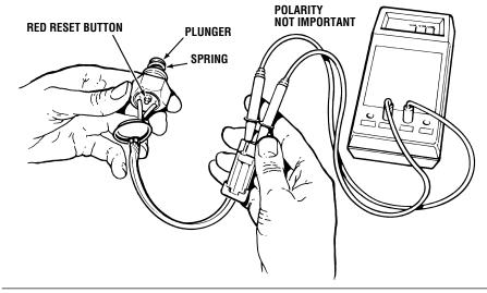
Figure 4-29. Overheat Sensor Test
