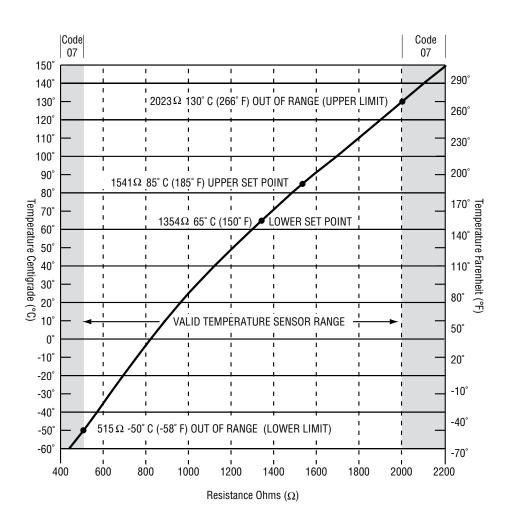
Figure 4-33. Coolant Temperature Sensor Graph
