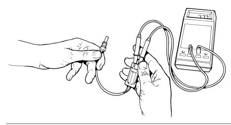
Figure 4-32. Temperature Sensor Test
