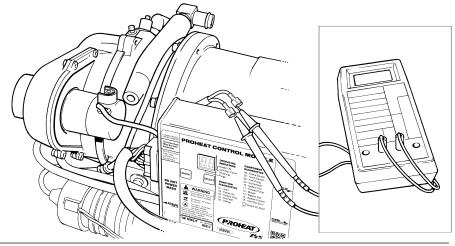
Figure 4-39. Hour Meter (Auxiliary Output) Test
