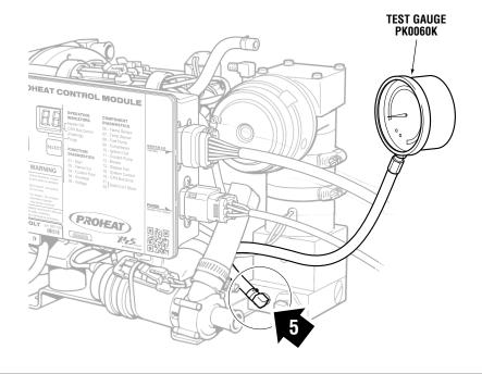
Figure 4-11. Installation of Test Gauge
