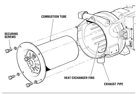
Figure 5-4. Heat Exchanger
