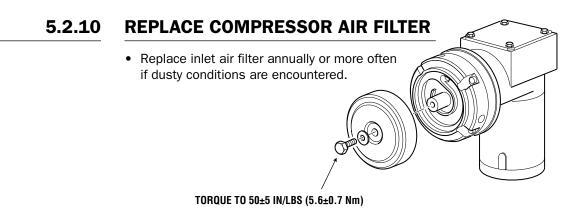
Figure 5-10. Compressor Air Filter
