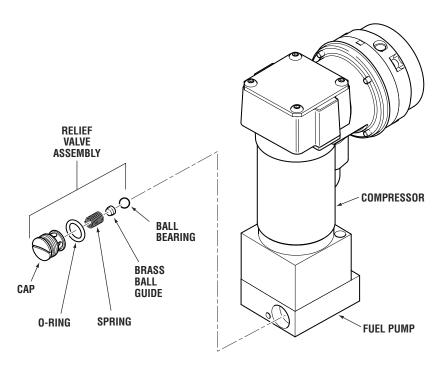
Figure 4-15. Pressure Relief Valve
