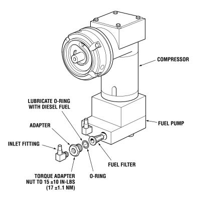
Figure 4-13. Check Valve Filter
