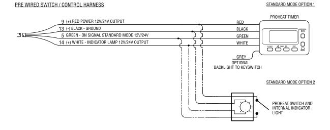
Figure 2-25. Pre wired switch/control harness
